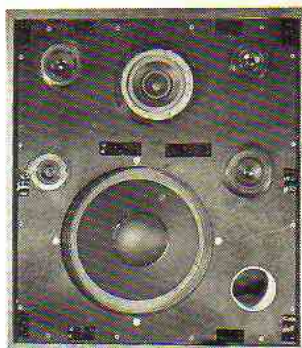
The Rectilinear III Lowboy design employs a ported enclosure with a 12-inch woofer, 5-inch mid-range, and four cone tweeters distributed over the front panel.
